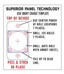
CAUTION-CHECK MEASUREMENT OF TEMPLATE PRIOR TO USE TO ASSURE THAT IT PRINTED ACCURATELY. THE CENTER OF THE TOP HOLE TO THE CENTER OF THE BOTTOM HOLE MUST BE 1.06".
